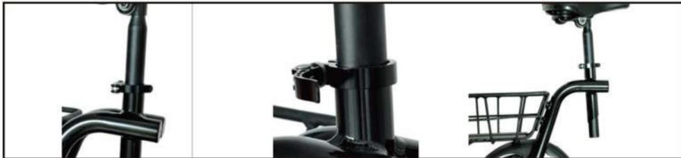
3. Open the quick-release on the seatpost on the frame and insert the seatpost. Adjust the seat height to a comfortable position, then close the quick release.
