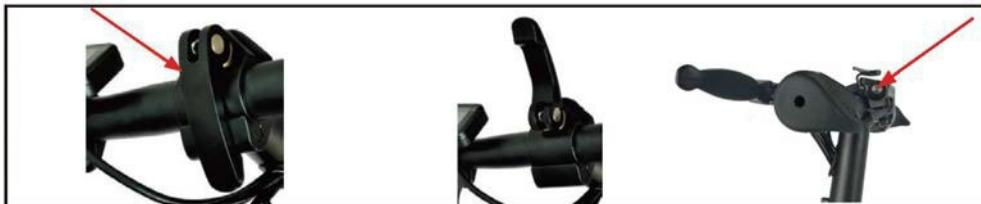
2. Open the quick-release in the middle of the handlebar and turn the handlebar to a position that is comfortable for you.
