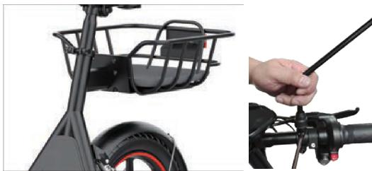
4. Remove the 4 screws securing the luggage basket above the rear fender. Adjust the luggage basket and attach
