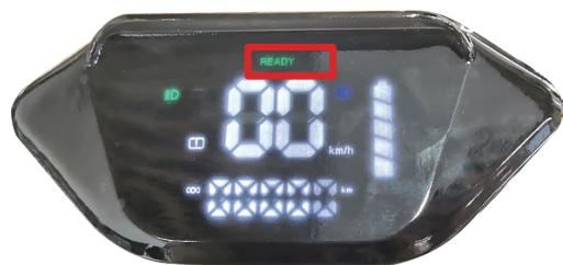
Insert the key into the power switch locked on the right handlebar, turn it in a clockwise direction, the display and the front light will turn on to indicate that the power has been connected.
