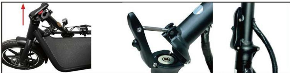
1. Take the folding electric scooter out of the box and pull the handlebar column locking lever forward and tilt the handlebars upwards. Then slide the locking lever backwards again.
