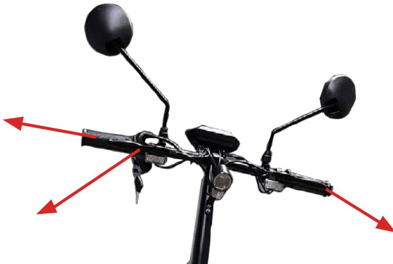
Use the throttle grip to accelerate. You can use the front and rear brakes to brake. You can choose from three speed levels.
